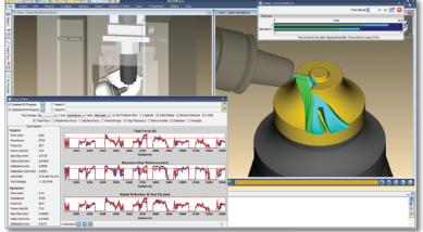
VERICUT is equipped with NC program optimization capabilities. Based on the cutting tool geometry, part material, and programmed cutting conditions, VERICUT automatically determines the optimum safe feed rate for each cut. The VERICUT optimized NC program will greatly improve cutter performance resulting in significant cycle time savings, reduced tool wear, improved tool life, and better finished parts.
