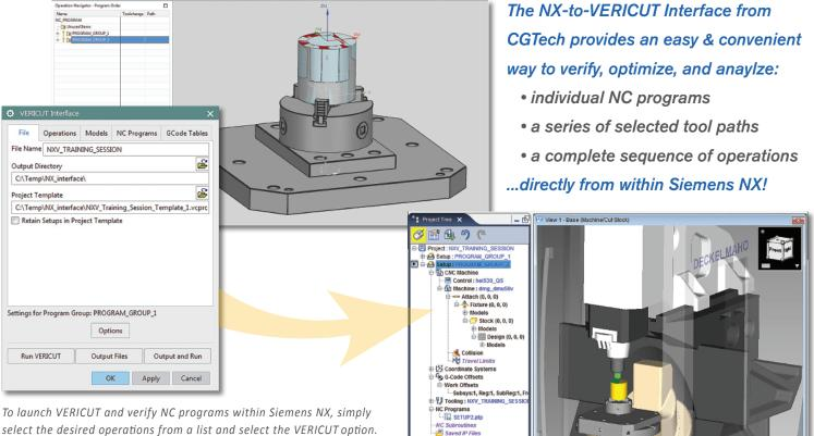
To launch VERICUT and verify NC programs within Siemens NX, simply select the desired operations from a list and select the VERICUT option. Settings from the Operations Navigator will be automatically transferred to VERICUT's Project Tree.
